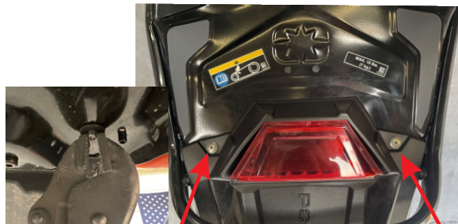
Drill out these 2 large flanged rivets and be sure to hold the back with a vise grip as shown.
