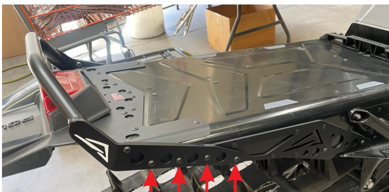
Drill 1/4" holes & install 6M x 20mm bolts here along with nyloc nuts.
